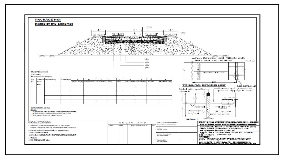
Figure 4: Typical Cross-Section of CC Road
