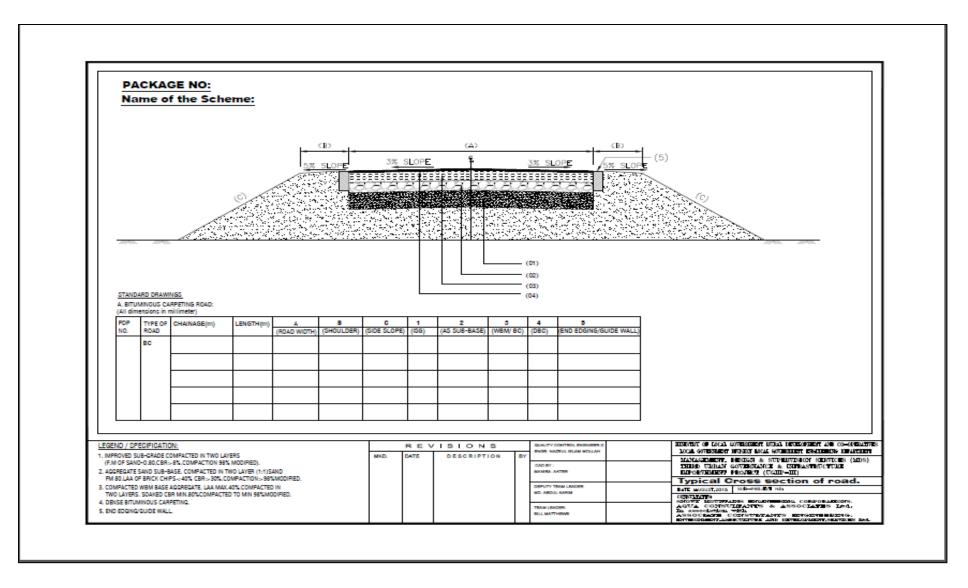
Figure 3: Typical Cross-Section of Bituminas Carpating Road
