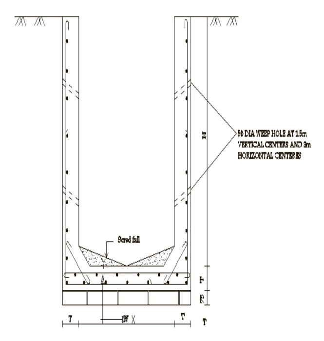
Figure 5: Typical Reinforced Cement Concrete U-drain
